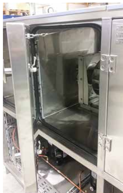
50mm Access door with compression T-handle and self gripping door sealing
